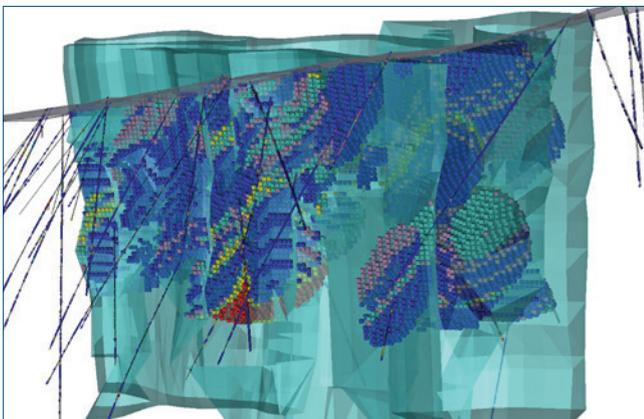
GEMS showing complex geological solid and block modelling based on drillhole and topographic mapping.
